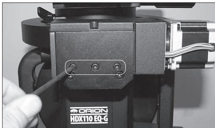
Fig. 7: Completely remove the three cosmetic cover screws on the front plate and set them aside.
